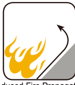
Reduced Fire Propagation NF C32-070-2.2(C1) IEC60332-3-24 EN50266-2-4
